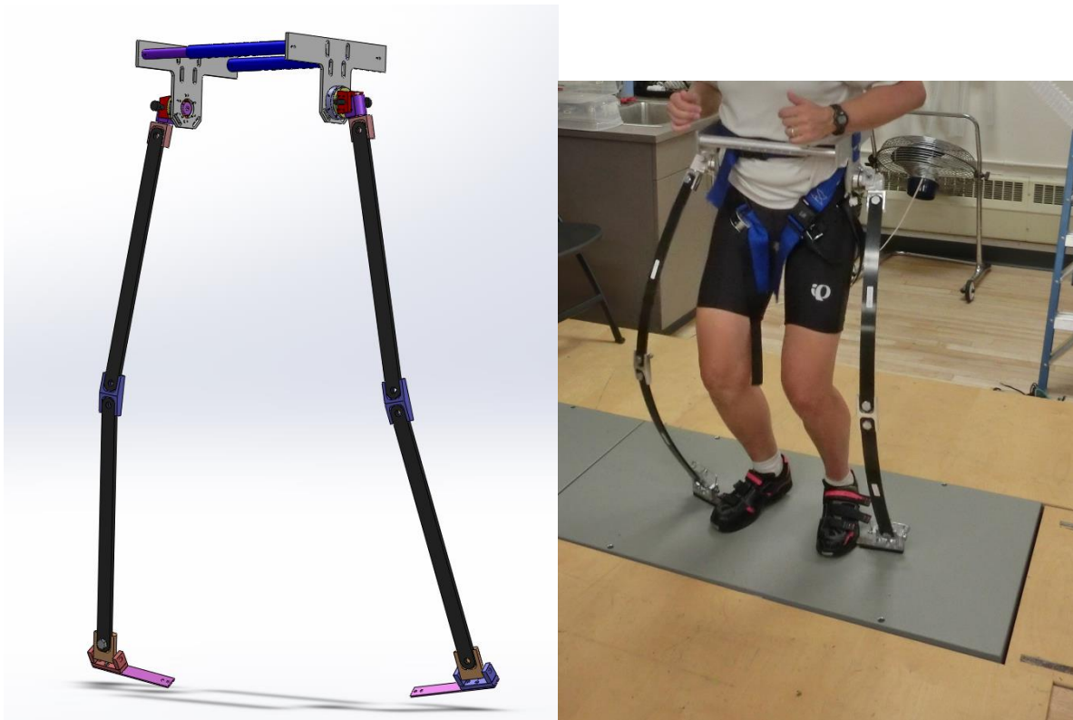
Figure 14. Progressively decreasing stiffness mechanism CAD model and in use.
