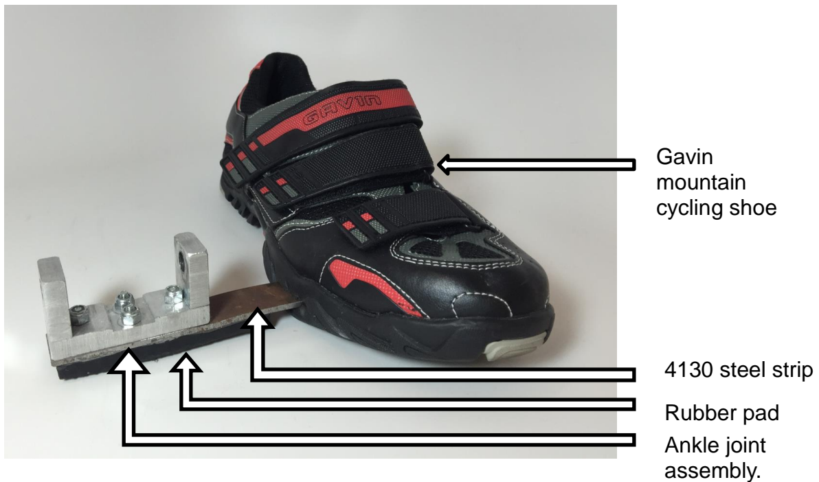
Figure 12. Gavin mountain cycling shoe with shoe attachment inserted into the sole, and bolts and screws present. A rubber pad has been adhered to the bottom of the spring steel plate, so that the bottom of the pad is even with the bottom of the sole when the shoe rests on the ground.
