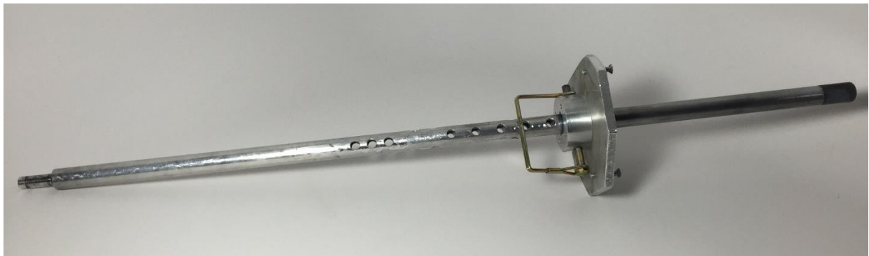
Figure 20. Upper (inner) telescoping rod. The hole arrays in the center are drilled to accommodate the varying leg lengths of exoskeleton users. In the final iteration, the spring compression plate has been trimmed on one side to avoid brushing against the user’s legs during hopping. Screws have been installed in the spring plate to guide the coil springs and prevent them from moving laterally during hopping. At right, the tip of the aluminum rod has been turned down, and a nylon bushing adhered in place to reduce the friction between the telescoping rods.
