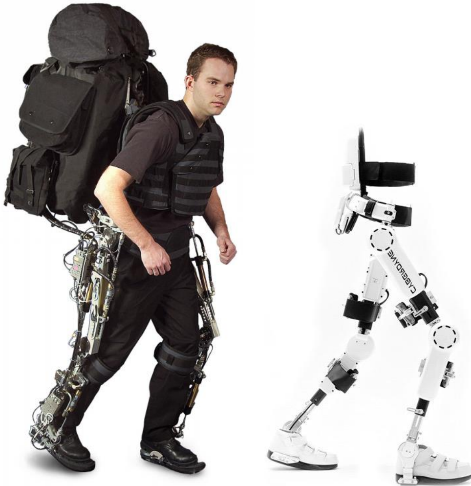
Figure 1. The Berkeley Lower Extremity Exoskeleton (left), and Cyberdyne’s HAL exoskeleton (right). Both of these exoskeletons assist human locomotion and are powered by a battery they house in their own structures, but they interact with their users in different ways. [A] [B]
