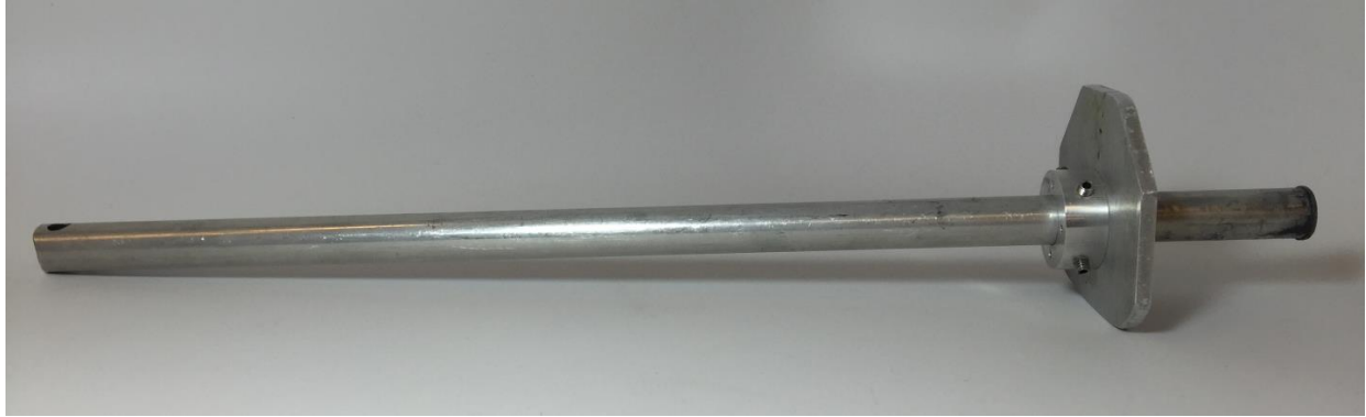
Figure 21. Lower (outer) telescoping rod. At left, the 0.375 inch hole has been drilled for the lynch pin of the ankle attachment assembly. At right, the inside diameter of the hollow aluminum rod has been widened. A nylon shoulder bushing has been adhered inside to reduce friction between the rods.
