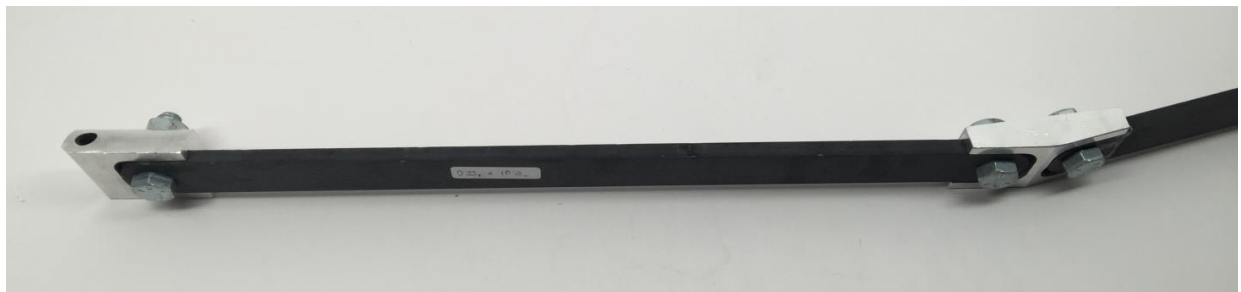
Figure 16. The bottom half of a bow spring, showing the knee joint (right), and the ankle joint (left).
