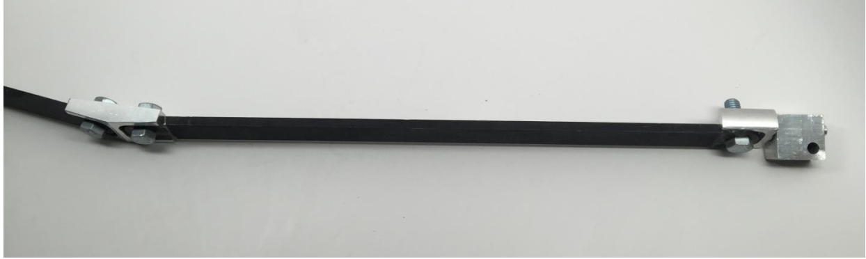
Figure 15. The top half of a bow spring, showing the knee joint (left), which holds the two bow springs at a 165-degree angle, and the assembled axial rotation shaft and abduction collar (right), which attach the bow spring to the hip and allow the leg to rotate. These two components are part of the hip joint assembly (Figure 10).
