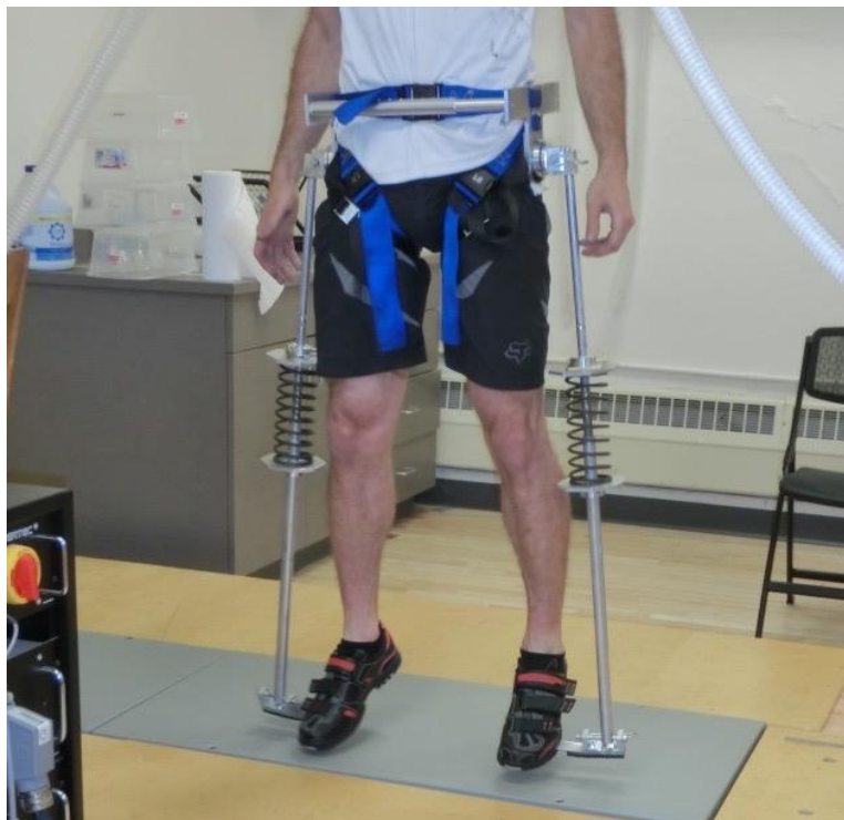
Figure 19. Coil spring assembly in use. The bow spring has been exchanged for the coil spring assembly; however, the same hip joint is used for both designs.
