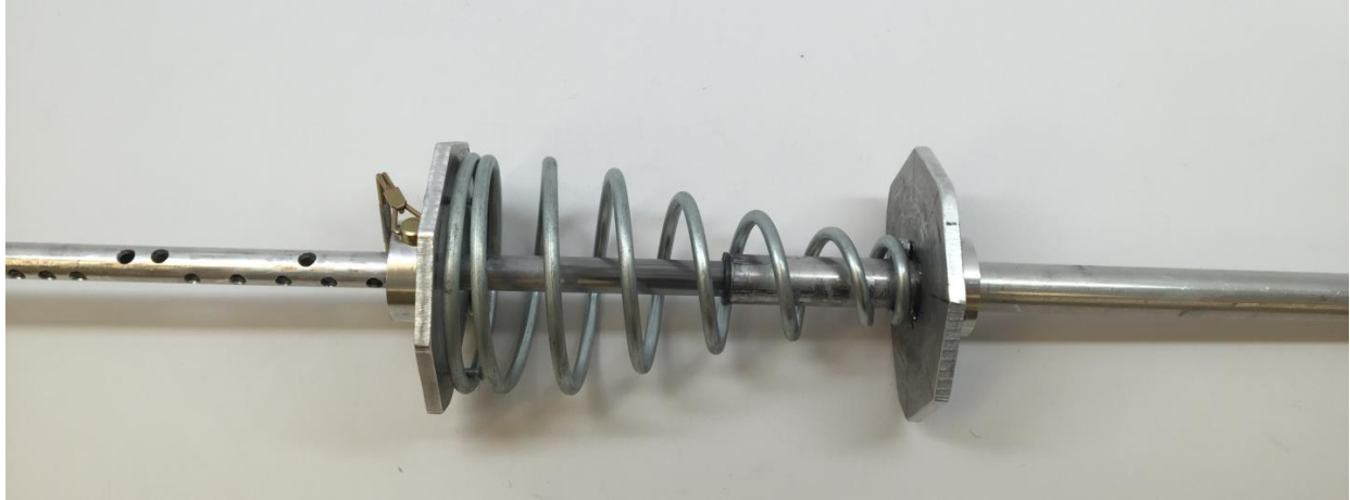
Figure 18. View of telescoping rods with conical coil spring. The two spring plates compress the coil spring between them as the telescoping rods are pressed towards one another.
